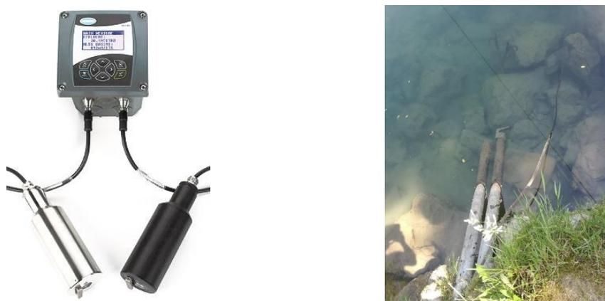
Figure 12 Turbidity sensor Solitax\_sc and SC1000 communication interface (left); sensor in a pipe on gauging station Suha on Sora River (right)
