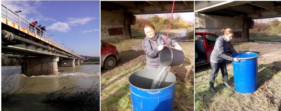
Figure 16 Integrated 200 litre water sample at gauging station Sava-Podsused
