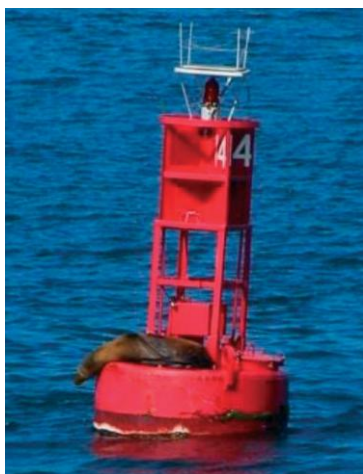
Figure 12: Buoy with an AIS AtoN base station (ref. IECDIS EG / VTT EG presentation 25 June 2015)
