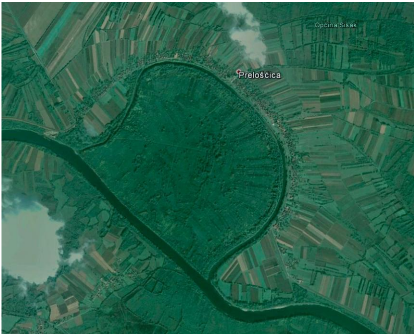
Figure 7: Cutoff example - Preloščica on the Sava River
