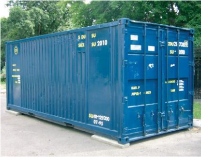
Figure 42: 20-feet (6.1 m) ISO container equals 1 TEU
