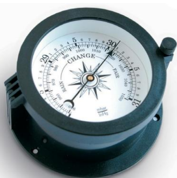
Figure 49: Modern metal aneroid barometers
