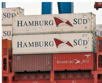
Figure 43: 40-feet container on the top of two 20-feet containers
