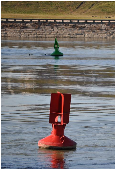
Figure 30: Red and green buoy with radar reflector for marking the fairway (Source: Plovput)
