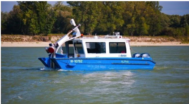
Figure 26: Multi-beam survey vessel on the Austrian Danube
