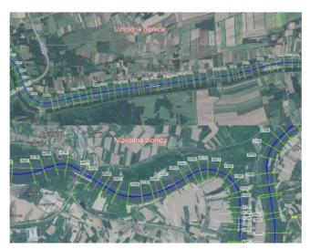
Figure 10: Groyne disposition for one-way navigation, sector "Jaruge –Novi Grad"
