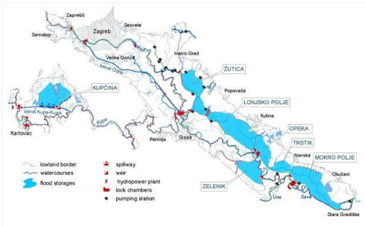
Figure Ap2-3: Rationalized flood control solution
