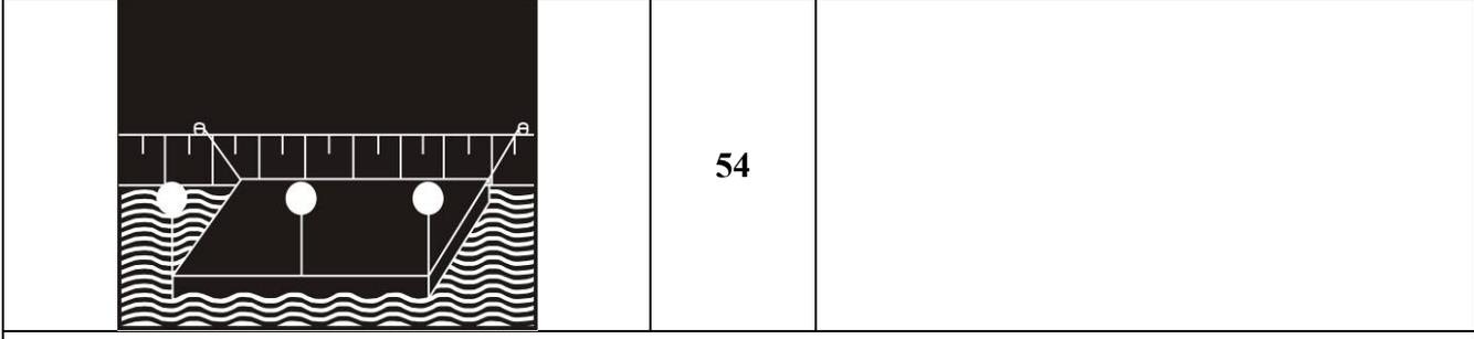
Article 3.23: Assemblies of floating material and floating establishments when stationary.
