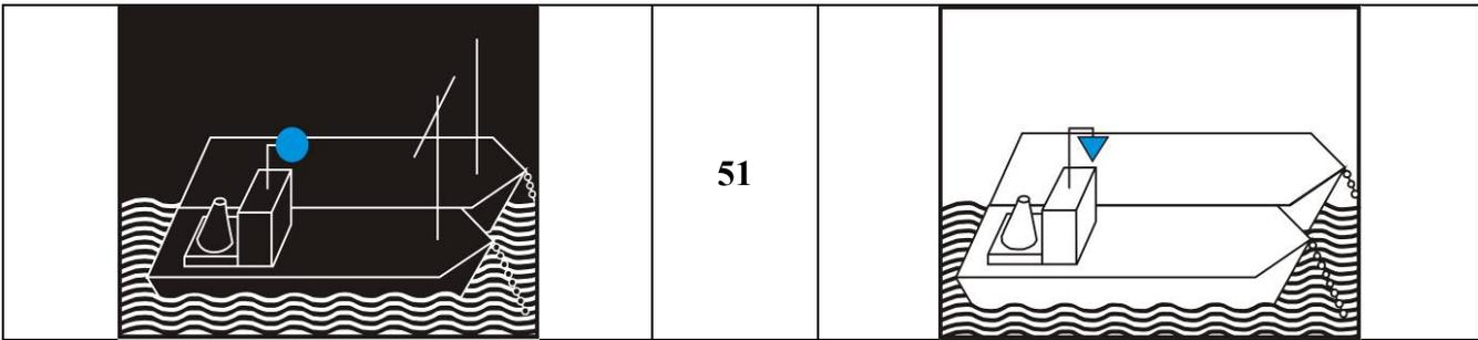
Article 3.21: Additional marking for stationary side-by-side formations carrying out certain transport operations involving dangerous substances.
