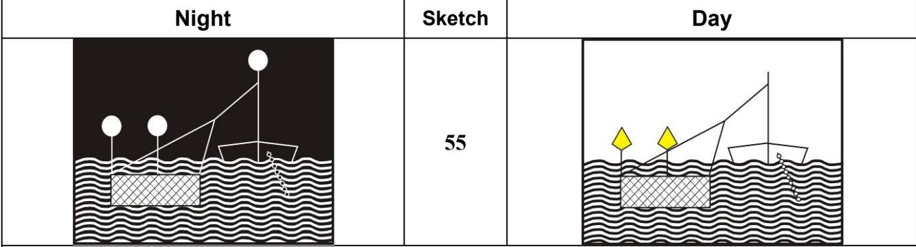
Article 3.24: Stationary vessels engaged in fishing with nets or poles.
