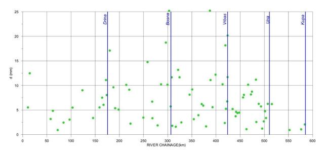
Figure 11 Longitudinal distribution of the Sava riverbed sediment diameter D50%
