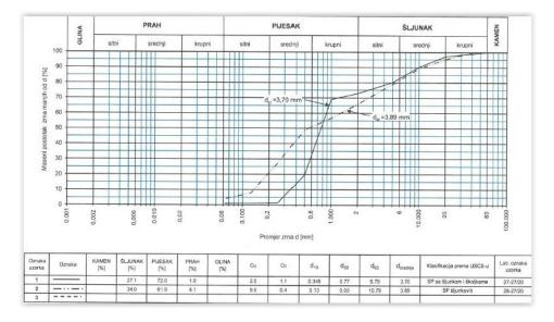
Figure 20 The bedload grain-size curve at g.s. Sava-Jasenovac in Sept 2020
