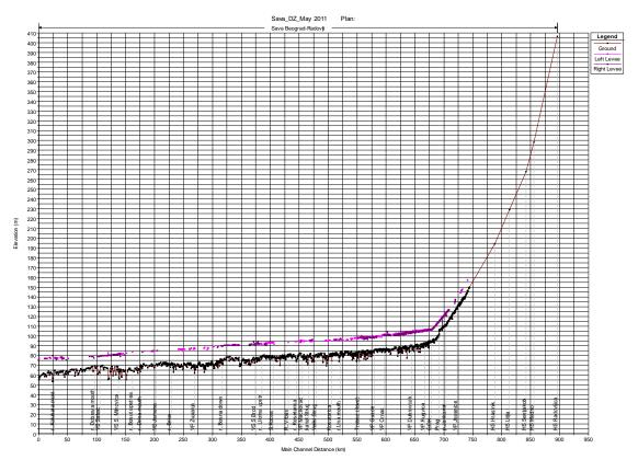
*Figure 7 The longitudinal profile of the Sava River between the mouth to the Danube (RS) and Radovljica (SI)*
