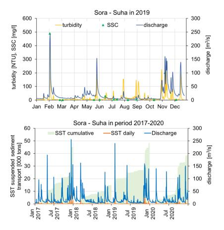
Figure 13 Mean daily discharge and turbidity together with periodic measurements of SSC (above) and daily and cumulative suspended sediment transport (below) at g.s. Suha on the Sora River
