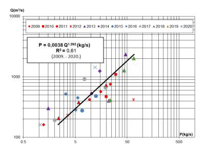
Figure 15 Sediment-rating curve for gauging stations Sava-Jasenovac in 2009-2020
