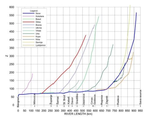
Figure 9 Schematic longitudinal profiles of the Sava River and its main tributaries
