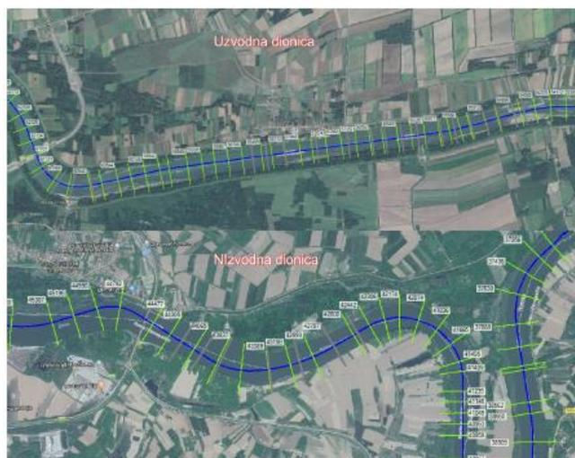
Figure 10: Groyne disposition for one-way navigation, sector „Jaruge –Novi Grad“
